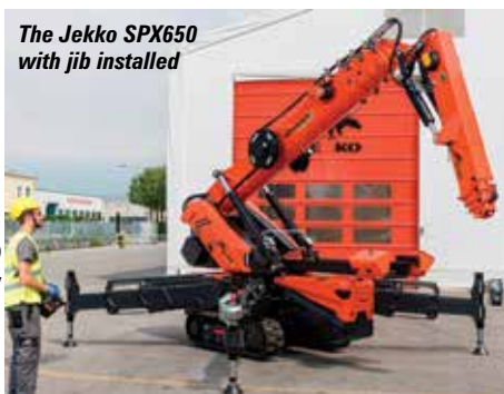
The Jekko SPX650 has a 23.5m tip height
