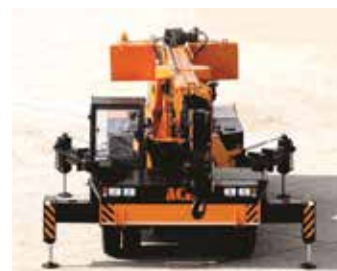
The addition of four outriggers allows it to double up as a 360 degree slewing crane.
