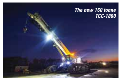
Maximum tip height for the TCC-1800 is 95.8m
