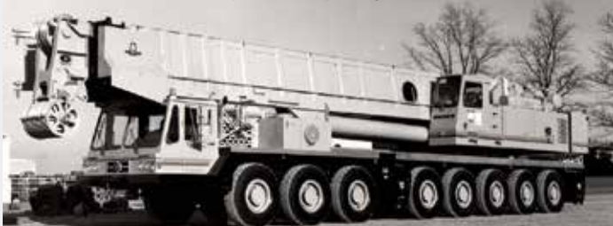
The Grove TM 2500 with Traplock boom pinning
